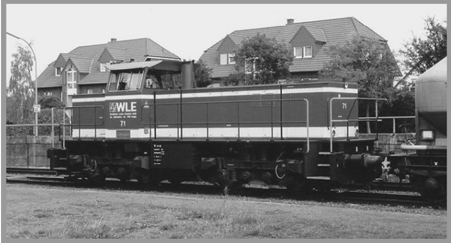
Diesellok #71, Named "Lippstadt" is a class G1204BB capable of producing 1120kW of power. Location: Erwitte, Germany, northbound toward Lippstadt.
